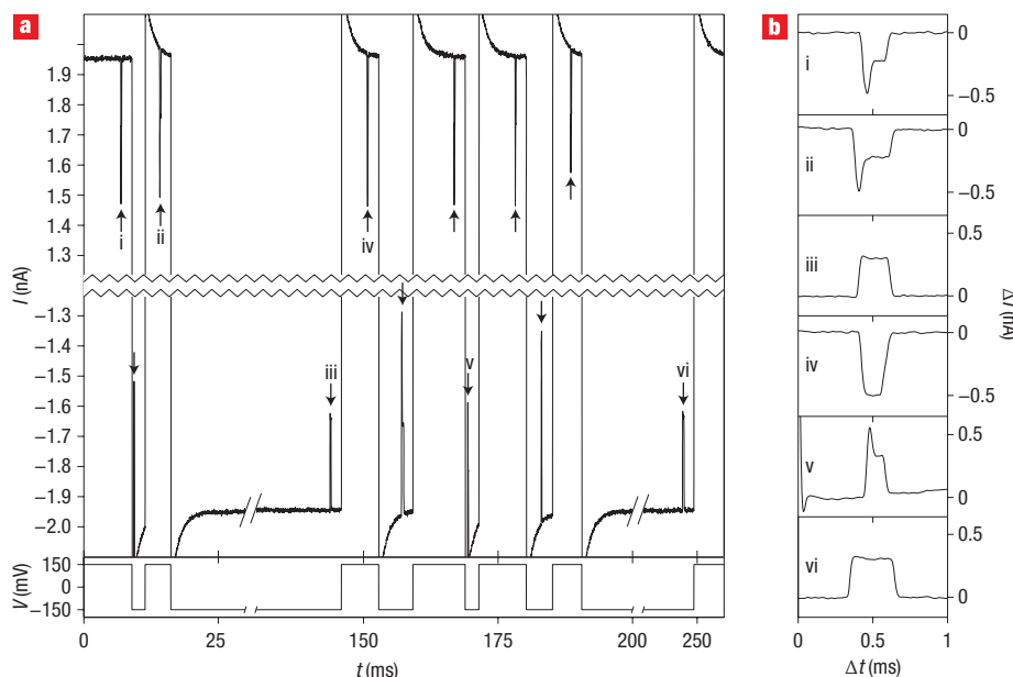
Figure 4 Current versus time traces from a single-molecule trapping experiment. a , A single 10 kbp dsDNA molecule passes the pore 12 times over 250 ms. The main panel shows the current through the pore versus time. For clarity, 2.4 nA are excised from the centre of the current axis, and the time axis has also been compressed. The short pulses (marked with arrows) show current being blocked as the molecule passes through the pore. At 2 ms after each passage, the voltage bias (plotted below the current) is reversed. As in Fig. 1, the molecule is initially captured at positive voltage bias. The exponential settling at the beginning of each transition results from charging of the membrane capacitance. b , Expanded current traces resulting from separate passages of the molecule through the pore. Each is labelled from i to vi to identify the portion of the current trace in a from which it was taken.
